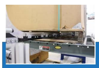
through the skid, secure the product and allow the product to be easily moved without strap interference. The H2B-PS fully automated pallet strapping machine is built around a heavy-duty steel frame to withstand the punishment of any environment. The Durable Construction of our equipment will streamline your packaging for many years to come.
