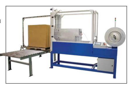
solution with its unique automated design capable of automatically strapping cases of finished goods or products onto a pallet or skid. What makes the H2B-PS unique is the ability to run the strapping lance
